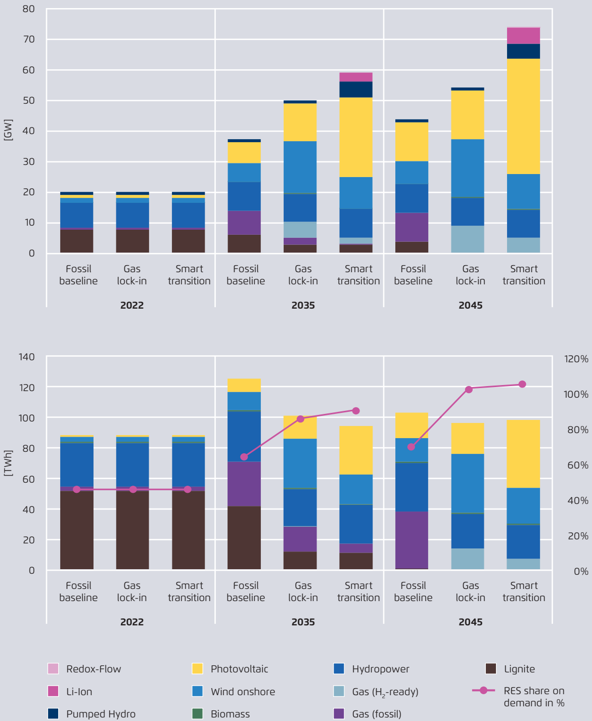
Installed capacities (top) and power generation (bottom) in 2022, 2035 and 2045 in the Western Balkans
