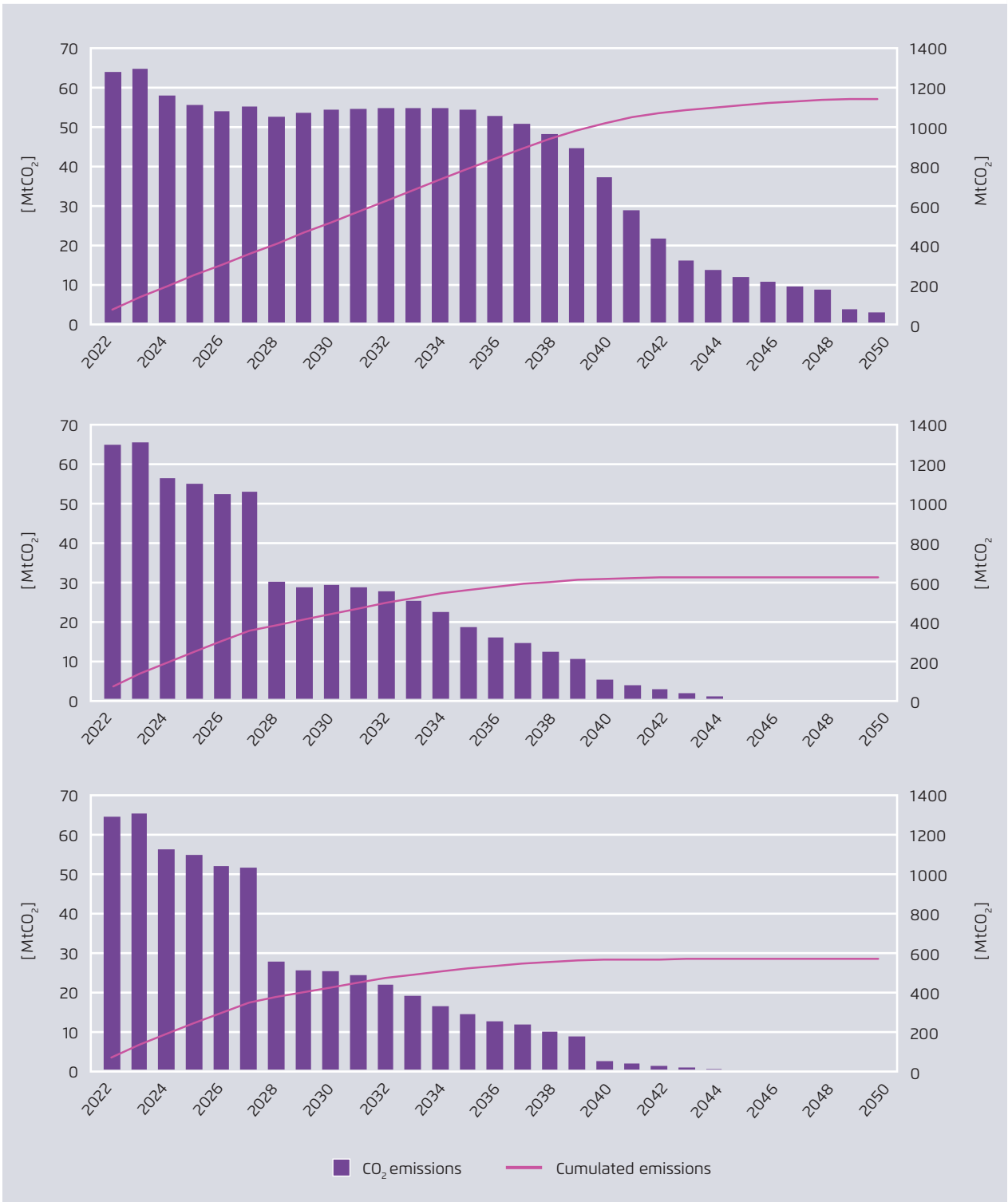
CO 2 emissions and cumulated CO 2 emissions in fossil baseline (top), gas lock-in (center) and smart transition (bottom) between 2022 and 2050
