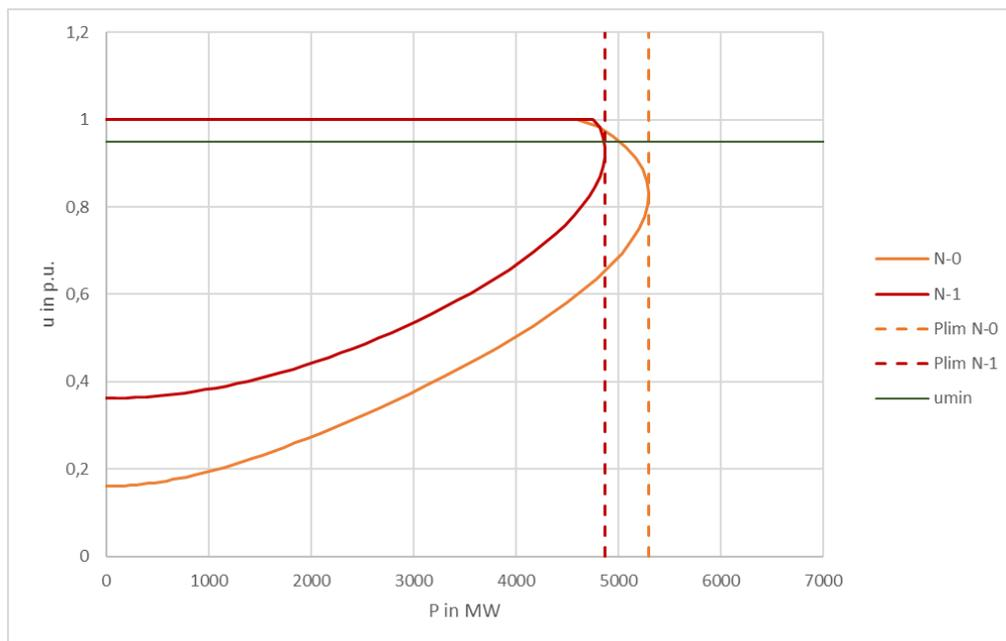
Figure 15: P-V-curve: high reactive power capability
