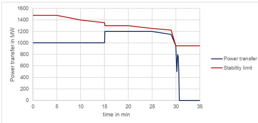
Figure 18: Long-term voltage instability caused by increased power transfer and reduced transfer limit (generic example).
