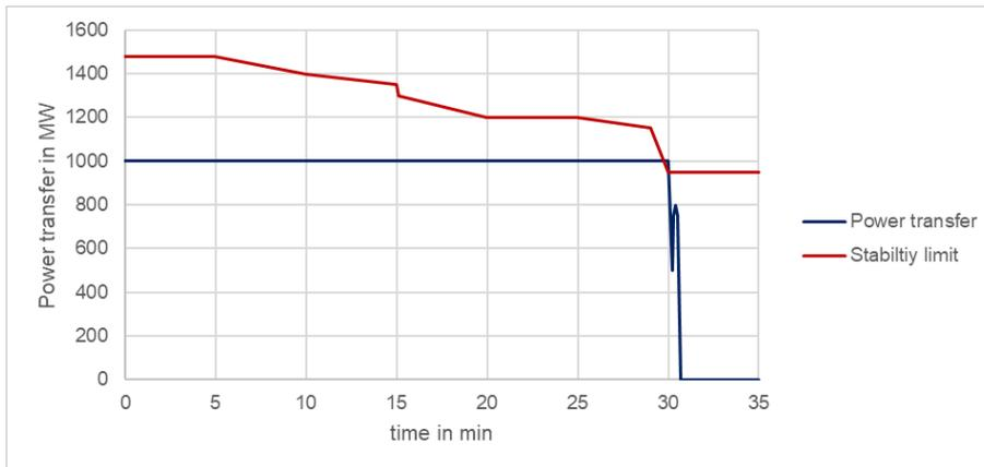
Figure 17: Long-term voltage instability caused by a reduced transfer limit (generic example).
