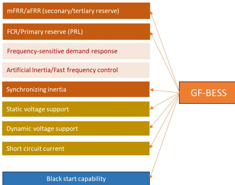
Figure 40: System services that BESS with grid forming converters can provide
