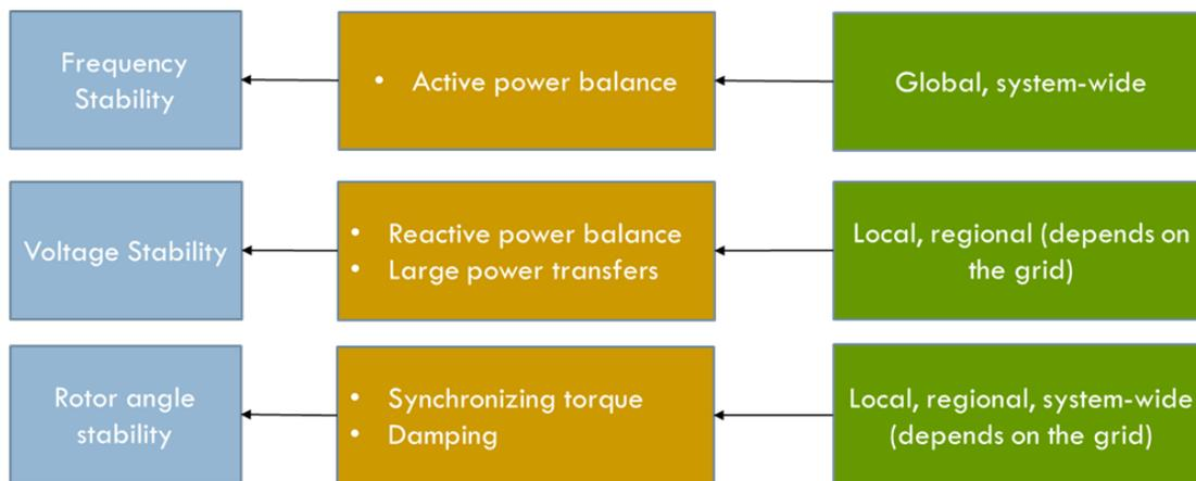
Figure 5: Most important stability phenomena in power systems according to CIGRE/IEEE [1]
