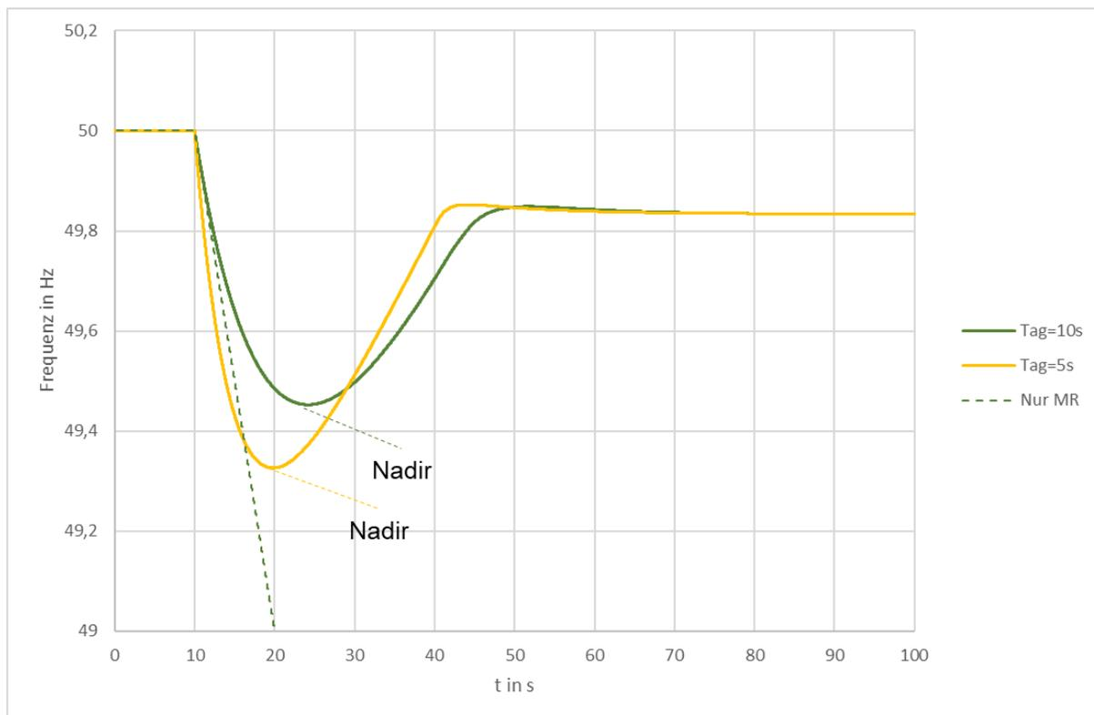
Figure 7: Frequency drop following a generator outage in function of system inertia (equivalent acceleration time constant): green: larger inertia, yellow: small inertia
