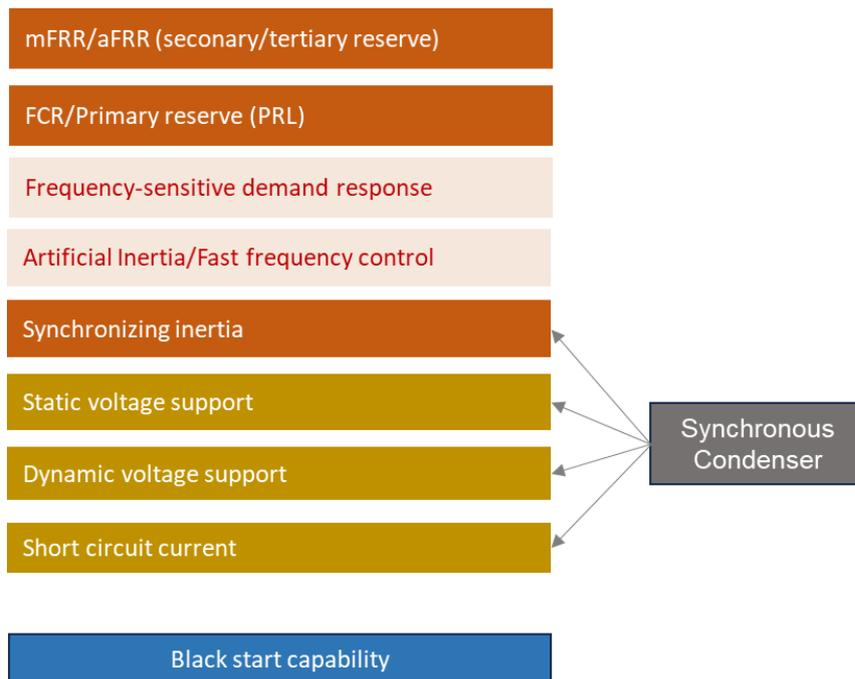
Figure 41: System services that synchronous condensers can provide
