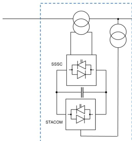
Figure 48: UPFC - Unified power flow controller
