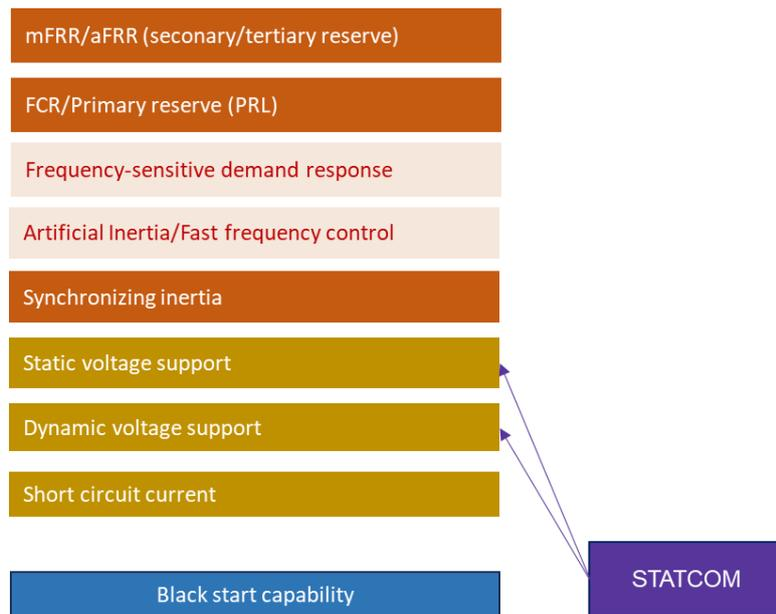
Figure 43: System services that STATCOMs can provide
