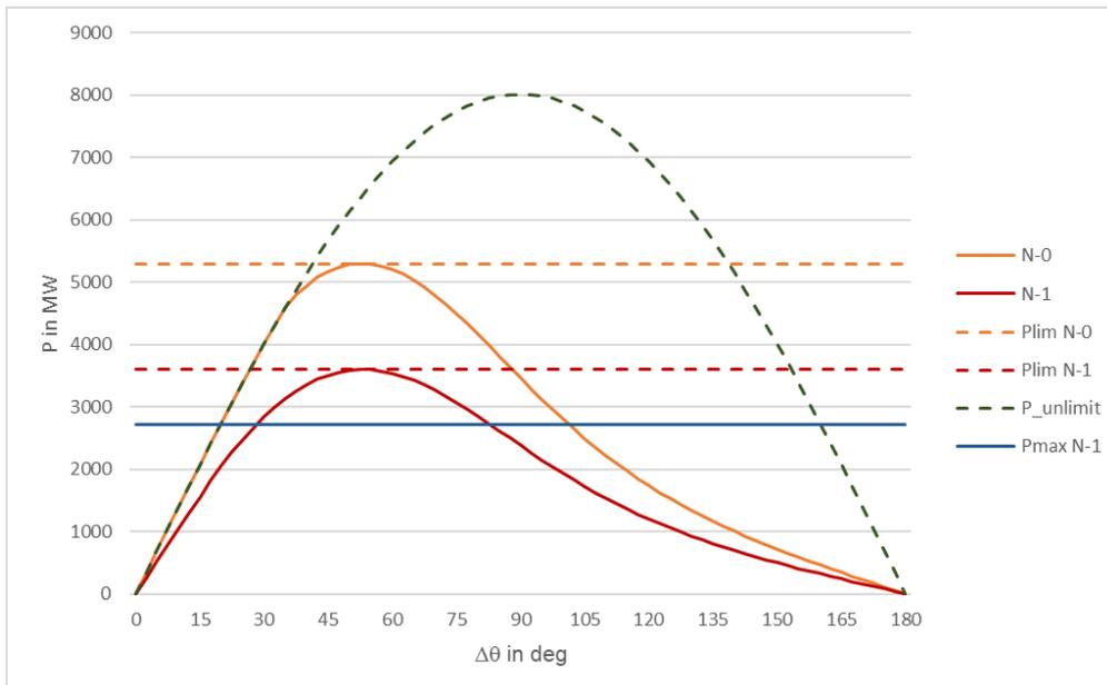
Figure 14: P- $\Delta\theta$ -curves and voltage stability limits
