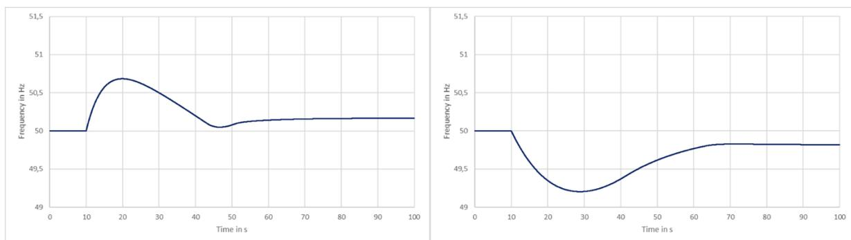
Figure 9: Frequency in area A1 (left) and area A2 (right) following a system split during a power transfer from A1 to A2
