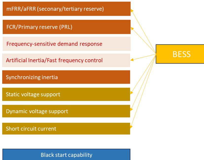
Figure 39: System services that BESS can provide
