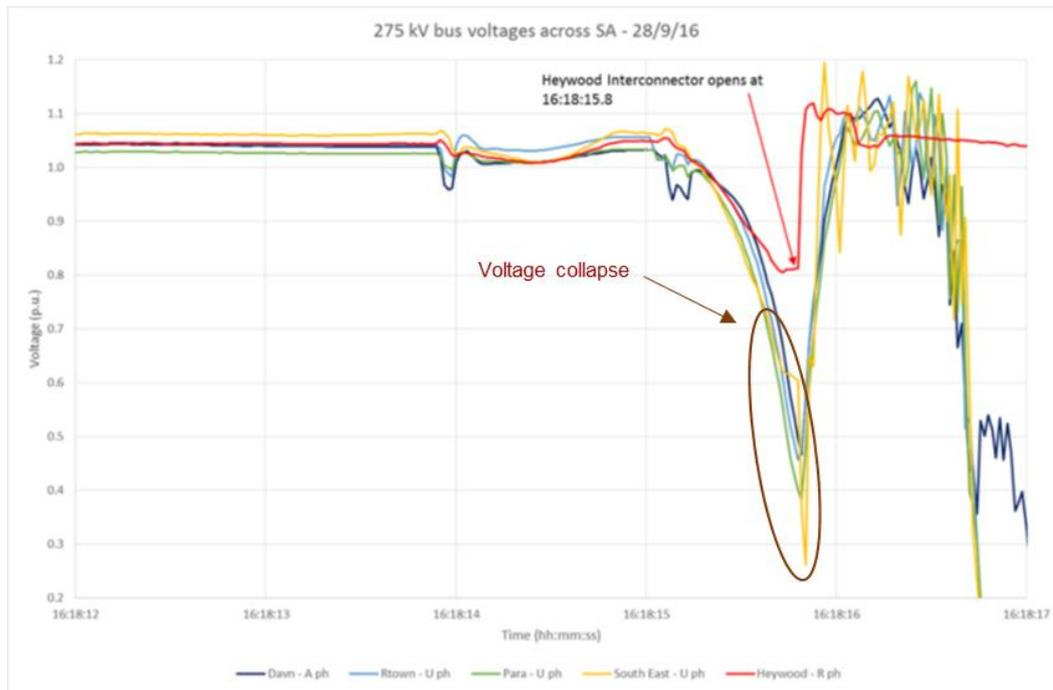
Figure 19: Voltages around the Heywood Interconnector/Australia, during the system black event in 2016 (taken from [20])
