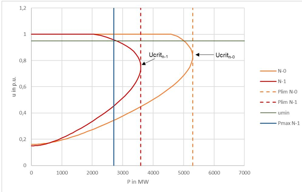
Figure 13: P-V-curves and voltage stability limits
