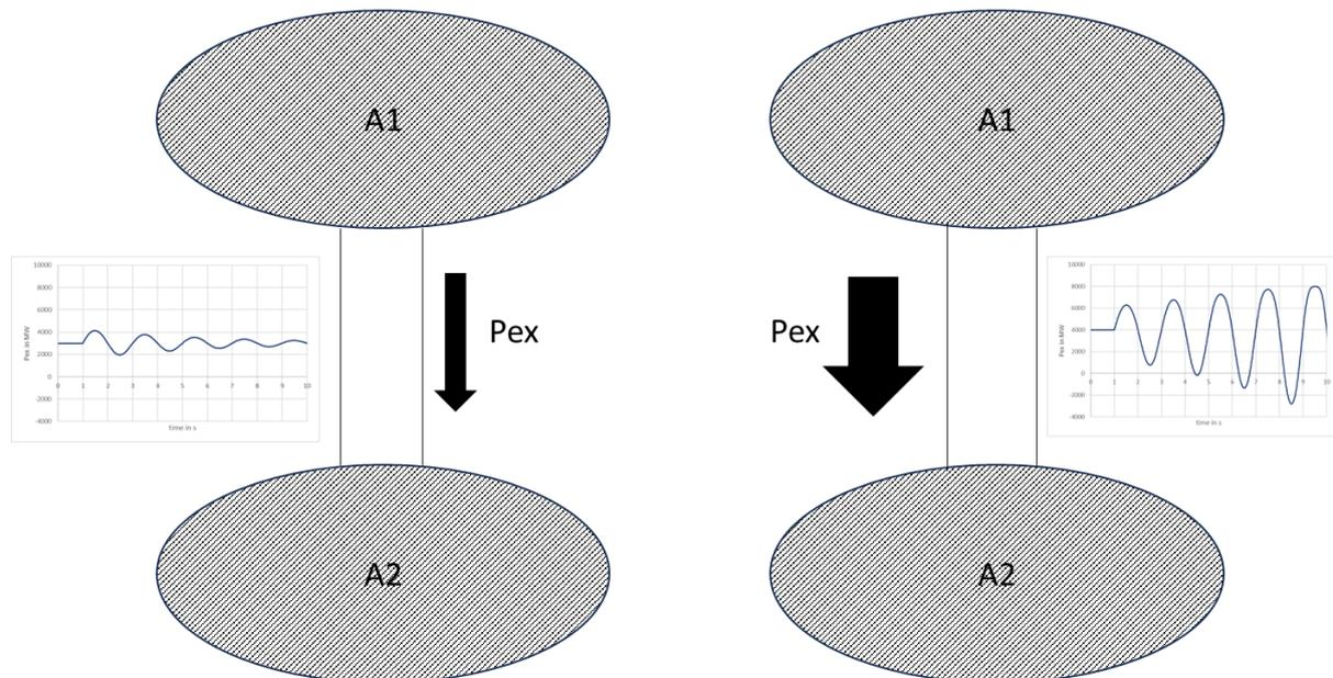
Figure 23: Inter area-oscillation with positive damping (left) and negative damping (right)
