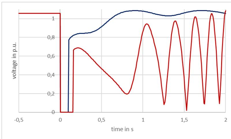
Figure 25: Voltage in p.u. (blue: stable, red: unstable)
