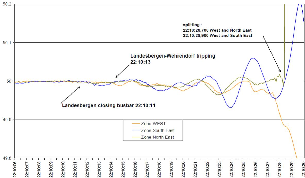
Figure 24: frequency recordings as retrieved by Wide Area Measurement Systems (WAMS) in the three areas from 22:09:30 to 22:20:00<sup>10</sup>
