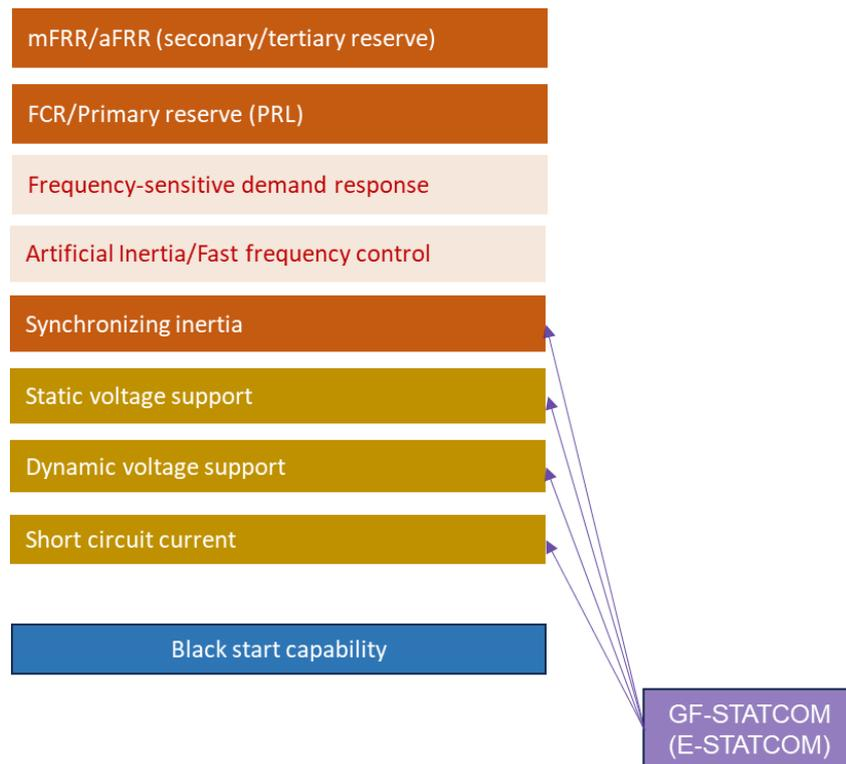
Figure 44: System services that E-STATCOMs can provide
