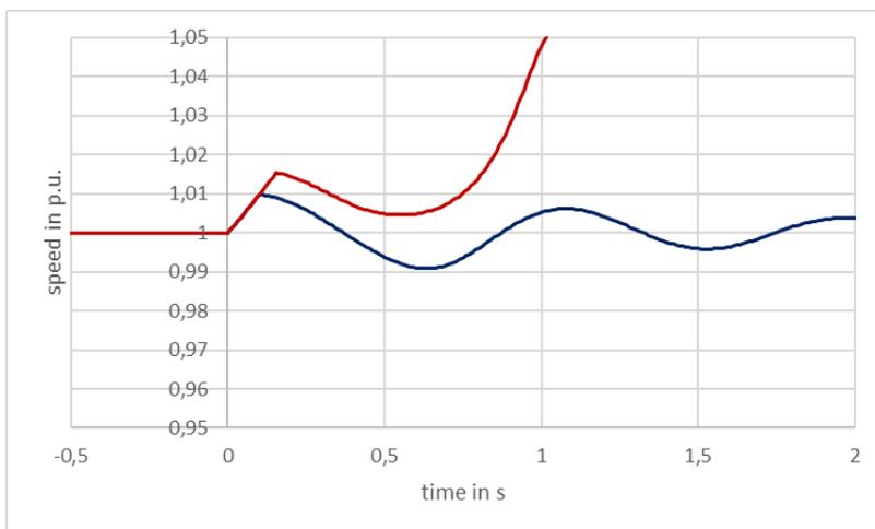
Figure 26: Generator speed (blue: stable, red: unstable)
