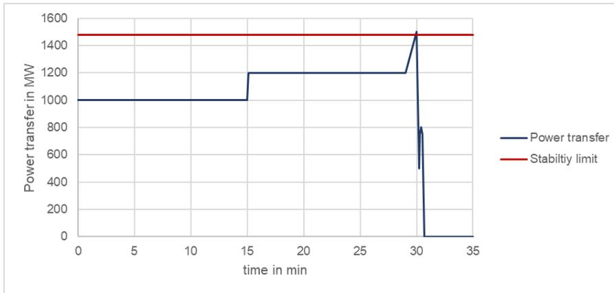
Figure 16: Long-term voltage instability caused by increased power transfer (generic example).
