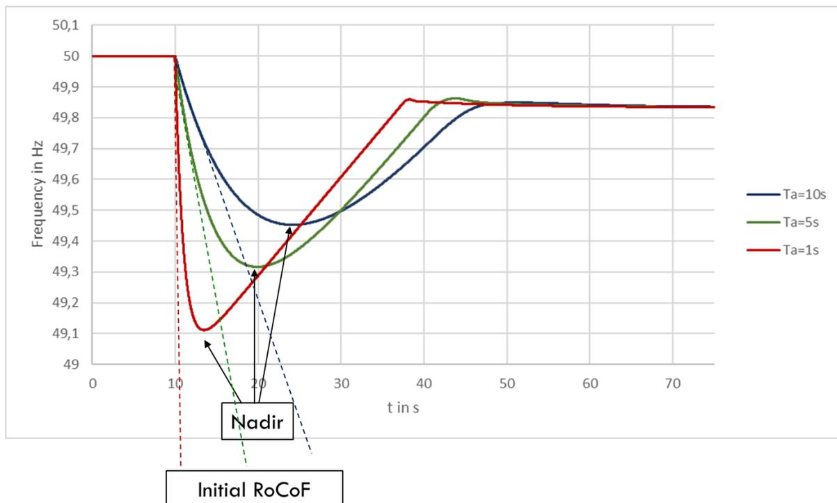
Figure 32: Frequency following a generator outage in function of the equivalent inertia of the system.
