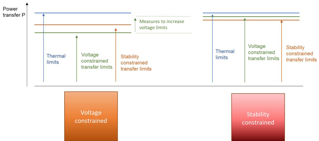
Figure 2: Stability constrained system (Stability limits below thermal and voltage limits)
