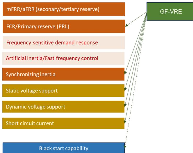
Figure 36: System services that VRE with grid forming converter can provide
