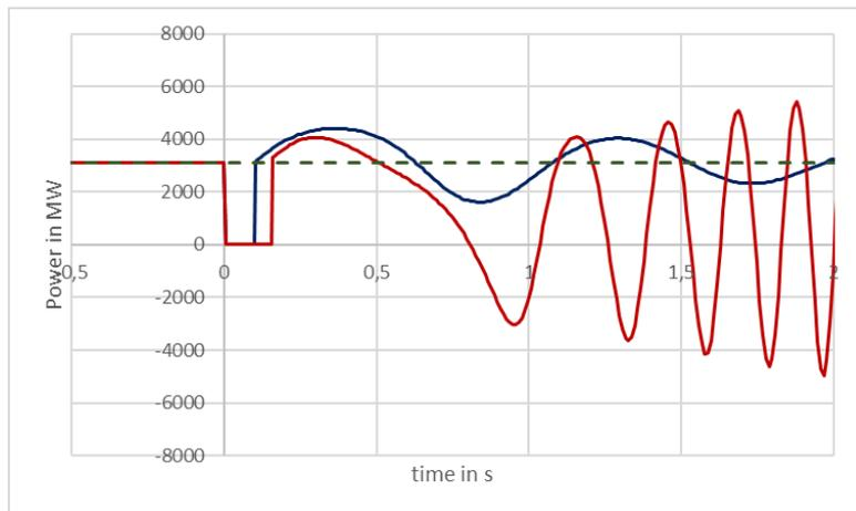
Figure 28: Power in MW (blue: stable, red: unstable)
