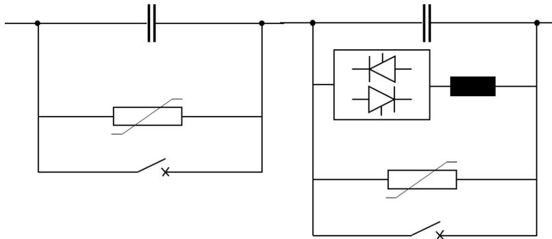
Figure 46: Thyristor-controlled series compensation (with protection equipment)
