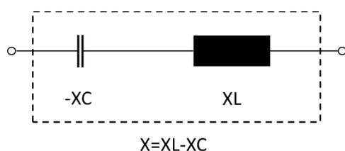
Figure 45: Static series compensator (passive, uncontrolled)
