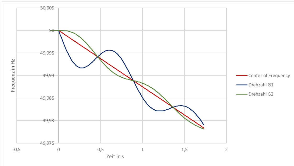
Figure 6: Centre of frequency with superposition of the local frequency at two different generator nodes.
