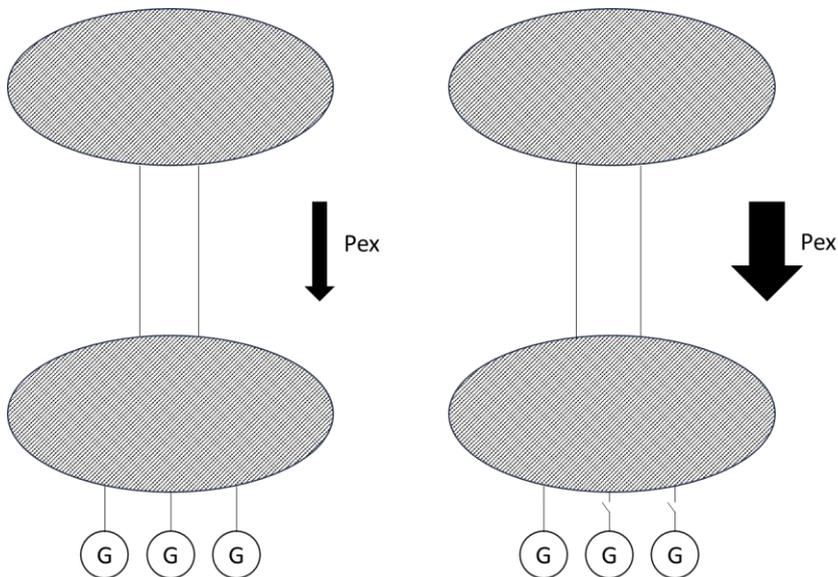
Figure 20: Disconnection of generators in an importing area resulting in increased power exchange.
