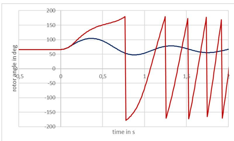
Figure 27: Rotor angle (blue: stable, red: unstable)
