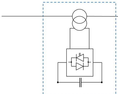
Figure 47: SSSC - Static Synchronous Series Compensator
