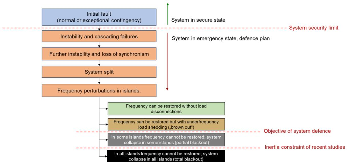
Figure 4: Series of stability events that can lead to major outages or system collapse.
