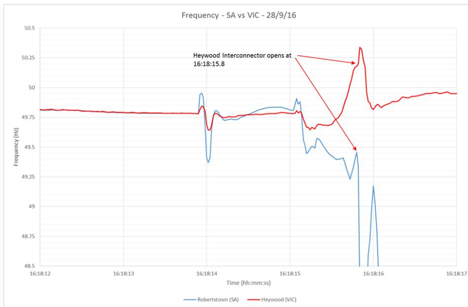
Figure 21: Frequency around the Heywood Interconnector/Australia, during the system black event in 2016 (taken from [20])
