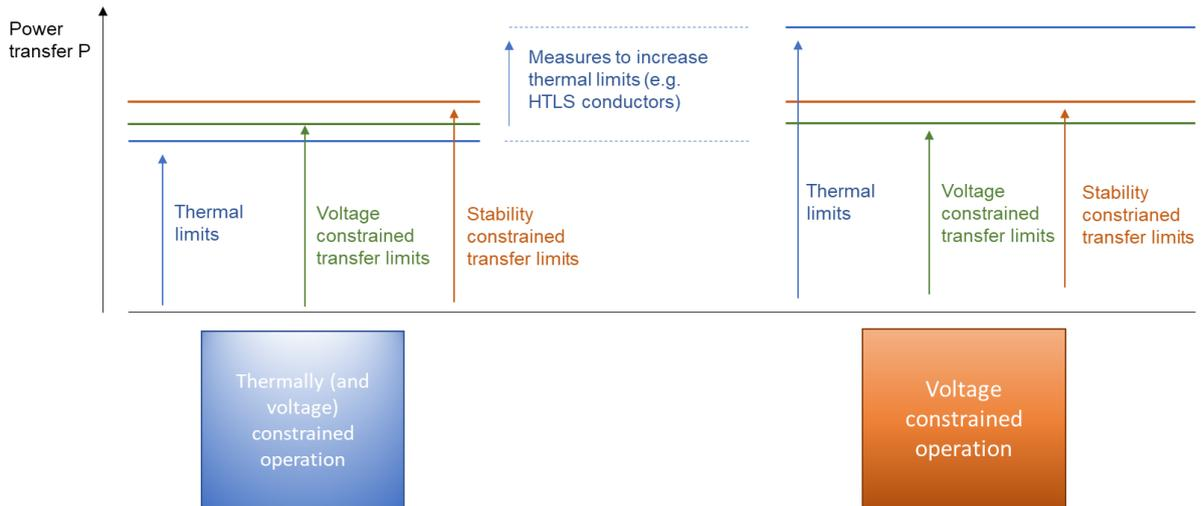
Figure 1: Thermally constrained and stability constrained operation
