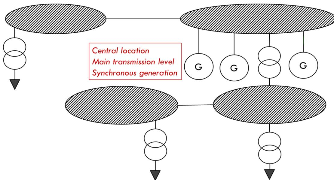
Figure 29: Conventional power system (supplied by large synchronous generators, which are close to the load centres)
