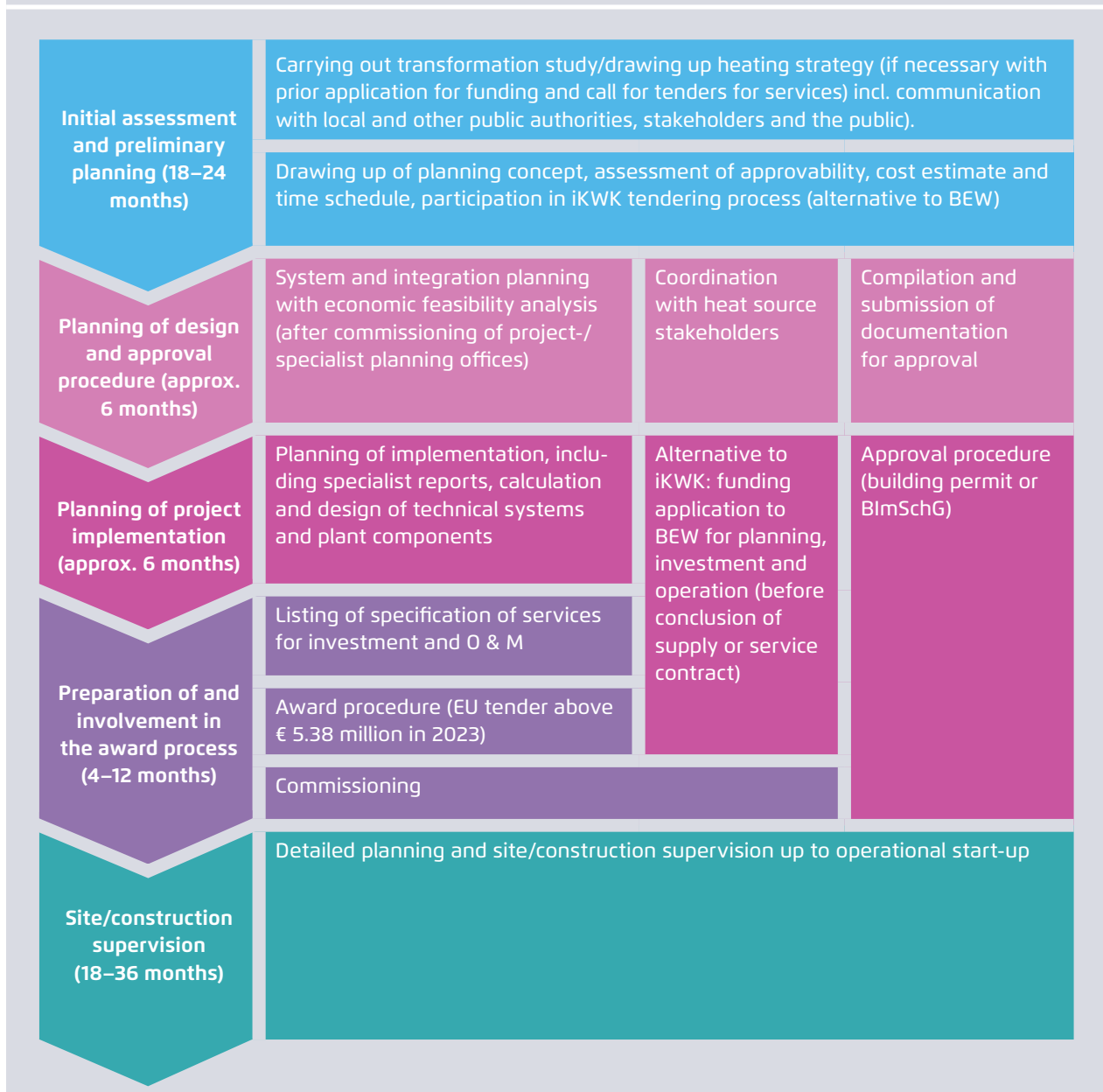
Phases of a large-scale heat pump project showing the most important tasks with approximate duration in months
