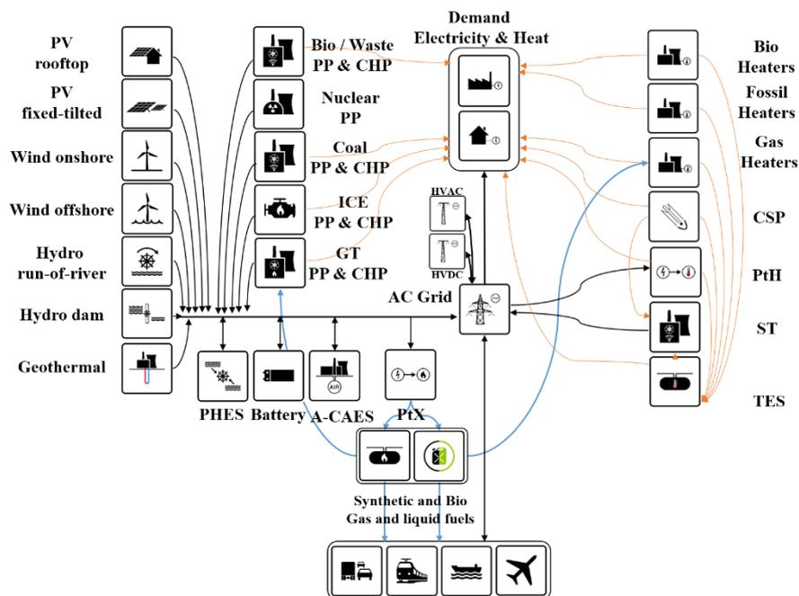
Figure 2.1: Schematic representation of the LUT Energy System Transition model. Abbreviations can be found in the Nomenclature section.
