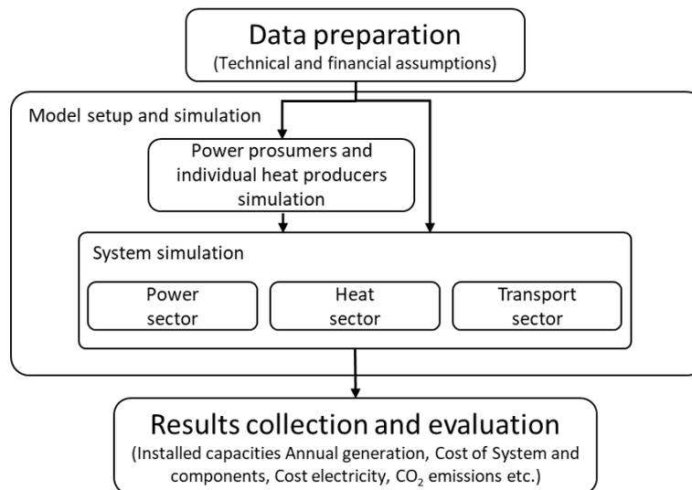
Figure A1: Fundamental structure of the LUT Energy System Transition model.
