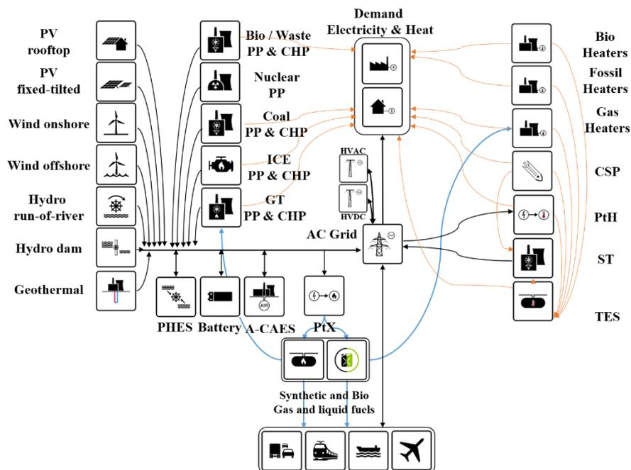
Figure A2: Schematic of the LUT Energy System Transition model comprised of energy converters for power and heat, storage technologies, transmission options, and demand sectors. Adapted from Bogdanov et al. [21].
