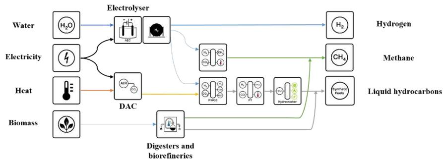
Figure A4: Schematic of the value chain elements in the production of sustainable fuels.
