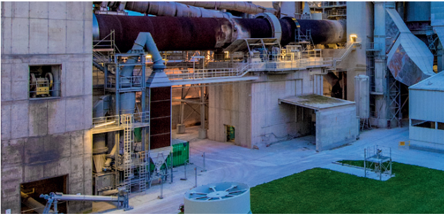
Pilot plant Oxyfuel clinker cooler, cement works Hanover, HeidelbergCement Photo: Steffen Fuchs, Heidelberg/Germany
