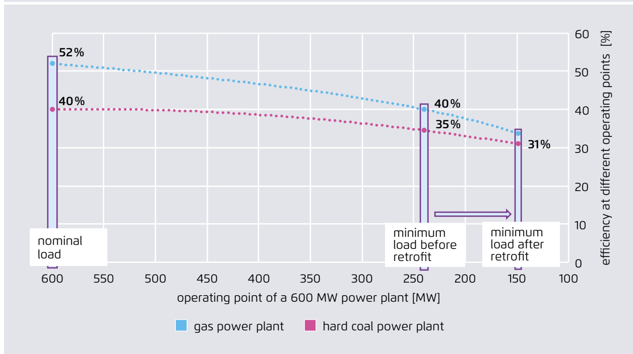
Relationship between plant output and efficiency of hard coal and CCGT gas power plants (600 MW nominal power) at different operating points (illustrative)
