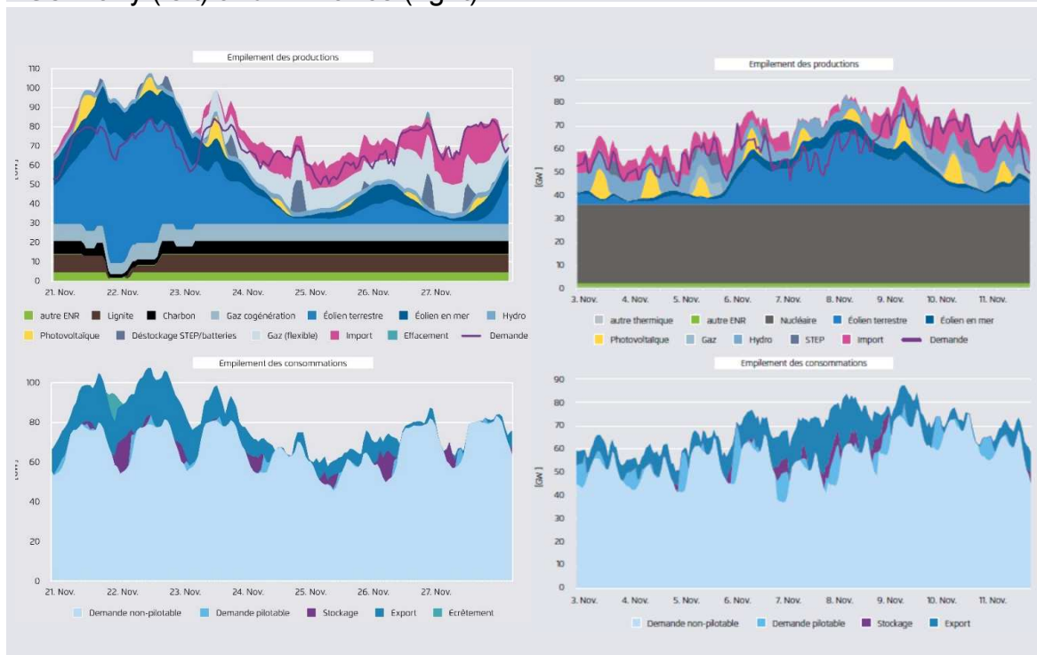
Production and consumption pattern during a week in November 2030 in Germany (left) and in France (right)*
