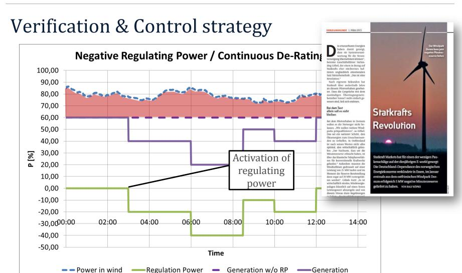
Continuous de-rating → losses in normal operation
