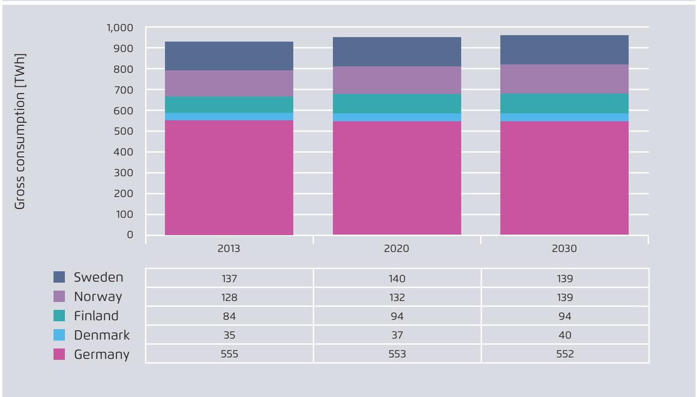
Projected electricity demand for individual countries (including grid losses but excluding own consumption on power plants, electricity consumption for district heat production (e.g. large heat pumps) and electricity consumption for pumped hydro storage).
