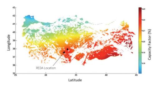
*Figure 14.* Capacity factor map of solar photovoltaic power plants (restricted locations eliminated)
