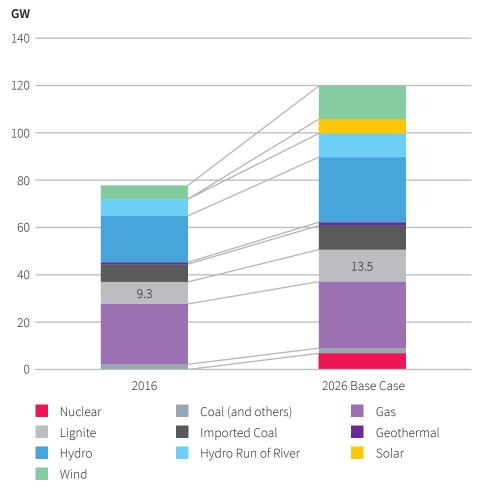
*Figure 16.* Total installed generation capacity in 2016 and 2026 according to the Base Case scenario
