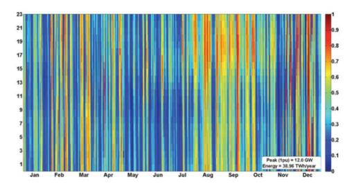
*Figure 88.* Times series power generation of wind power plants in 2026 (Per unit power generation based on maximum total power output by date and time for Base Case scenario, resource-driven)
