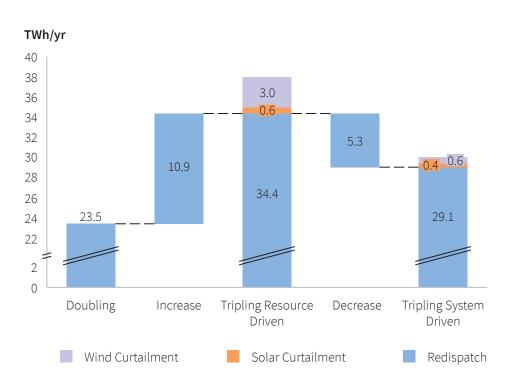
*Figure 51.* Comparison of redispatch and curtailment, resource-driven versus systemdriven strategy according to the Tripling scenario
