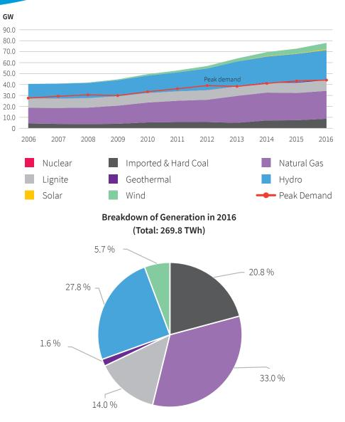
*Figure 7.* Breakdown of total installed capacity (top) and electricity generation (bottom) by source (2016)<sup>10</sup>
