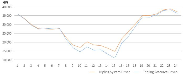
Figure 46. Net load deviation example; difference between resource-driven and system-driven strategies
