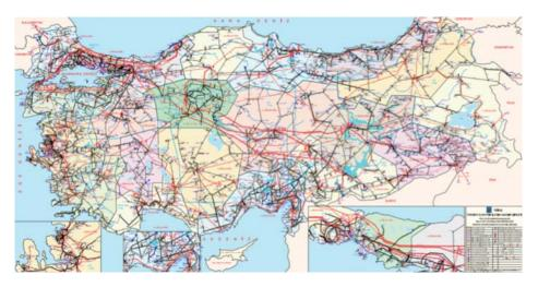
*Figure 71.* Map of high voltage transmission network, interconnections, thermal and hydropower plants (source: TEİAŞ)
