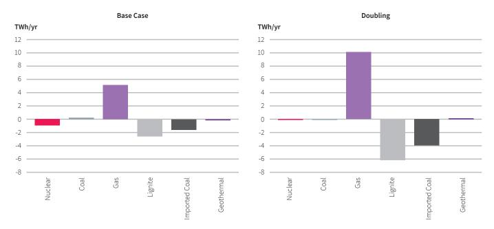
Figure 29. Changes in generation due to redispatch according to the Base Case and Doubling scenarios, 2026
