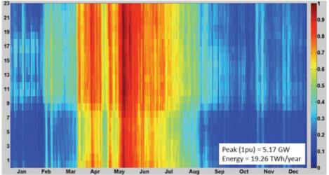
*Figure 92.* Times series power generation of run-of-river power plants, 2026 (8760 hours) (Per unit power generation based on maximum power output by date and time)
