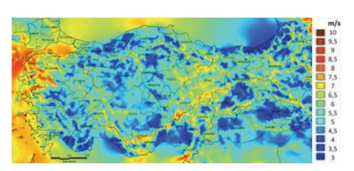
Figure 64. Wind speed atlas of Turkey (50 meters height and 200 meters resolution)
