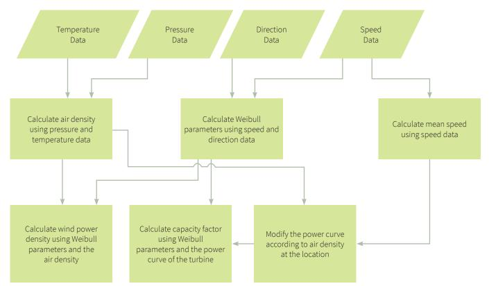
Figure 85. Methodology for estimating time-series wind power density of wind power plants<sup>174</sup>
