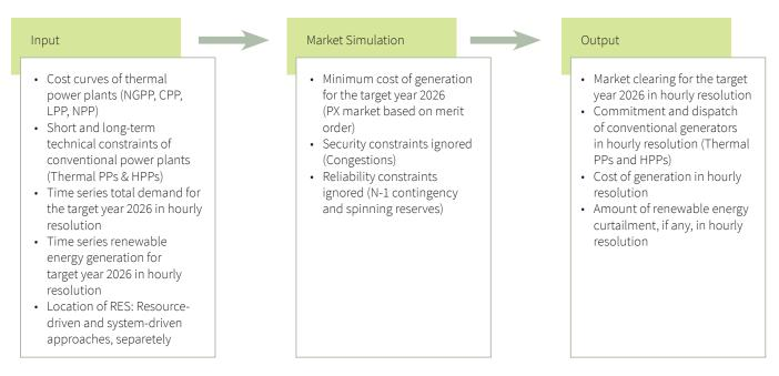
Figure 75. Key inputs and outputs of the market simulation
