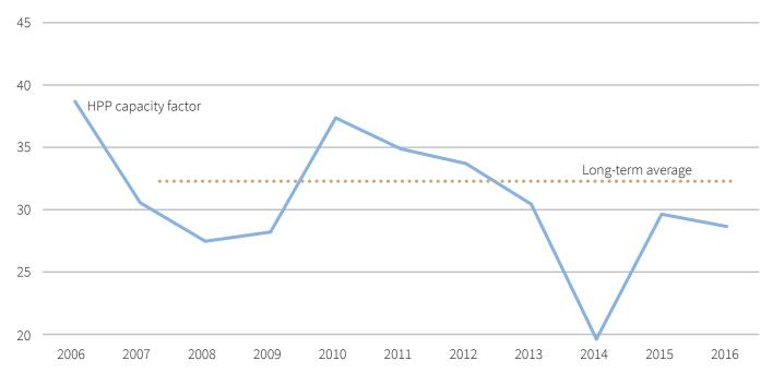
It should be noted that capacity factors<sup>128</sup> for hydro generation vary considerably yearby-year as seen in *Figure 63*<sup>129</sup>, due to varying precipitation levels (snow and rainfall); in this regard, 2016 can be considered as an average year.
