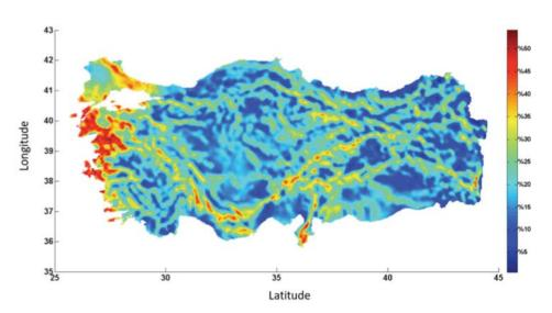
Figure 86. Wind capacity factor map determined based on the methodology
