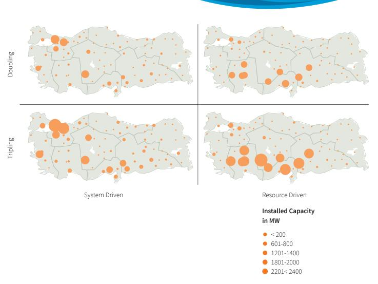
Figure 41. Comparison of solar capacity allocation in the resource-driven and system-driven strategies, 2026
