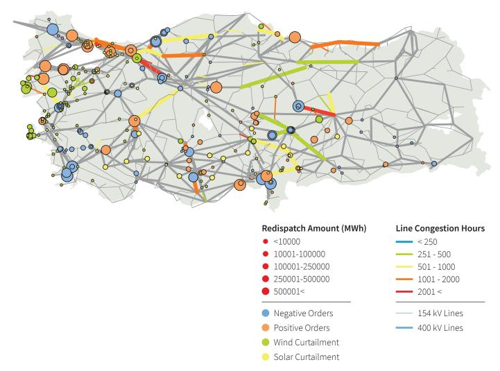
Figure 39. Annual congestion levels and thermal re-dispatch orders after transmission grid investments according to the Tripling scenario, 2026
