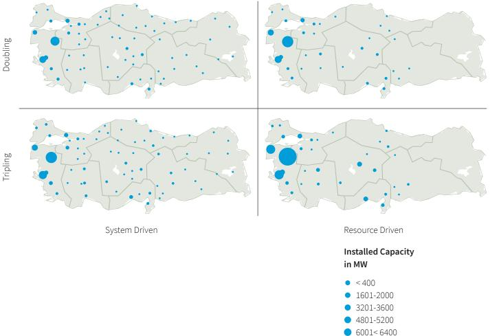
Figure 40. Comparison of wind capacity allocation in the resource-driven and system-driven strategies, 2026
