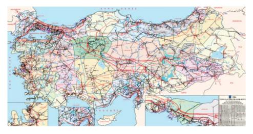
**Figure 8.** *Map of high voltage transmission network, interconnections, thermal and hydropower plants (source: TEİAŞ)*
