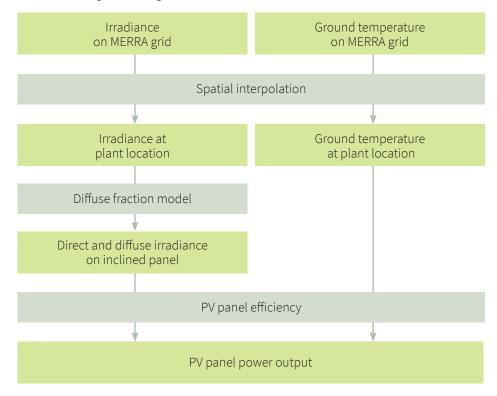
Figure 89. Overview of the approach used to model PV power output
