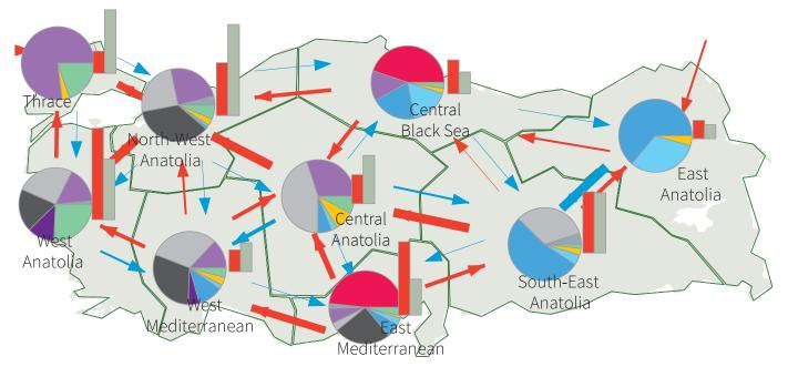
Figure 19. Regional generation/load balance and inter-regional exchange according to the Base Case scenario, 2026
