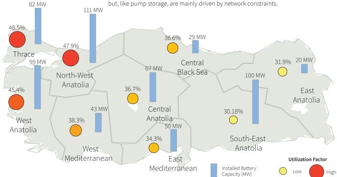
Figure 52. Regional distribution of capacity and capacity factors of battery storage
