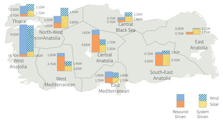
*Figure 42.* Allocation of wind and solar capacities in the resource-driven and system-driven strategies according to the Doubling scenario, 2026
