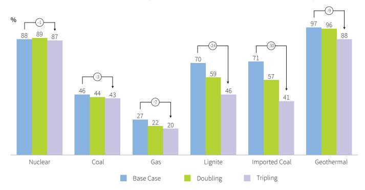
Figure 32. Capacity factors by source, Base Case, Doubling and Tripling scenarios, 2026
