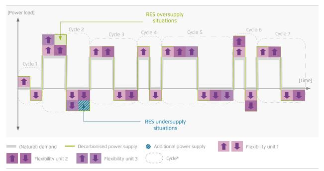
Agora Energiewende based on Consentec GmbH (2025); \*Cycle: One sequence of "charging" in oversupply situation and "discharging" in undersupply situation and, hence, thereby covering demand
