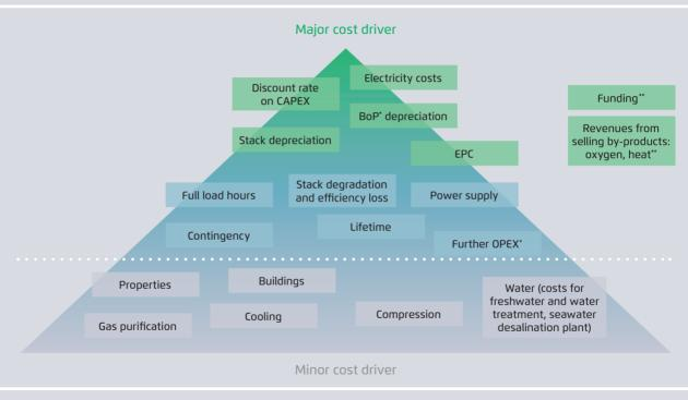
Umlaut (2023). \*Generic term. BoP: There is no standard definition of BoP, but it typically includes power supply, water conditioning, and process utilities like pumps, process-value-measuring devices, and heat exchangers. \*Despite their importance in real projects, the revenues from the sale of oxygen and heat as well as funding are not included in the consideration as they are not cost components.
