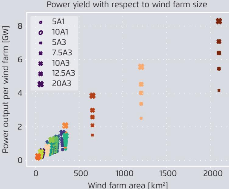
The colours represent the wind farm in accordance to Figure 10. The scenario is indicated by the symbol and symbol size as indicated by the legend on the top left. Larger wind farms generate more, but the effect is not directly proportional, i.e. a doubled area does not double generation. Similarly, larger installed capacity densities for a given wind farm generate more power.
