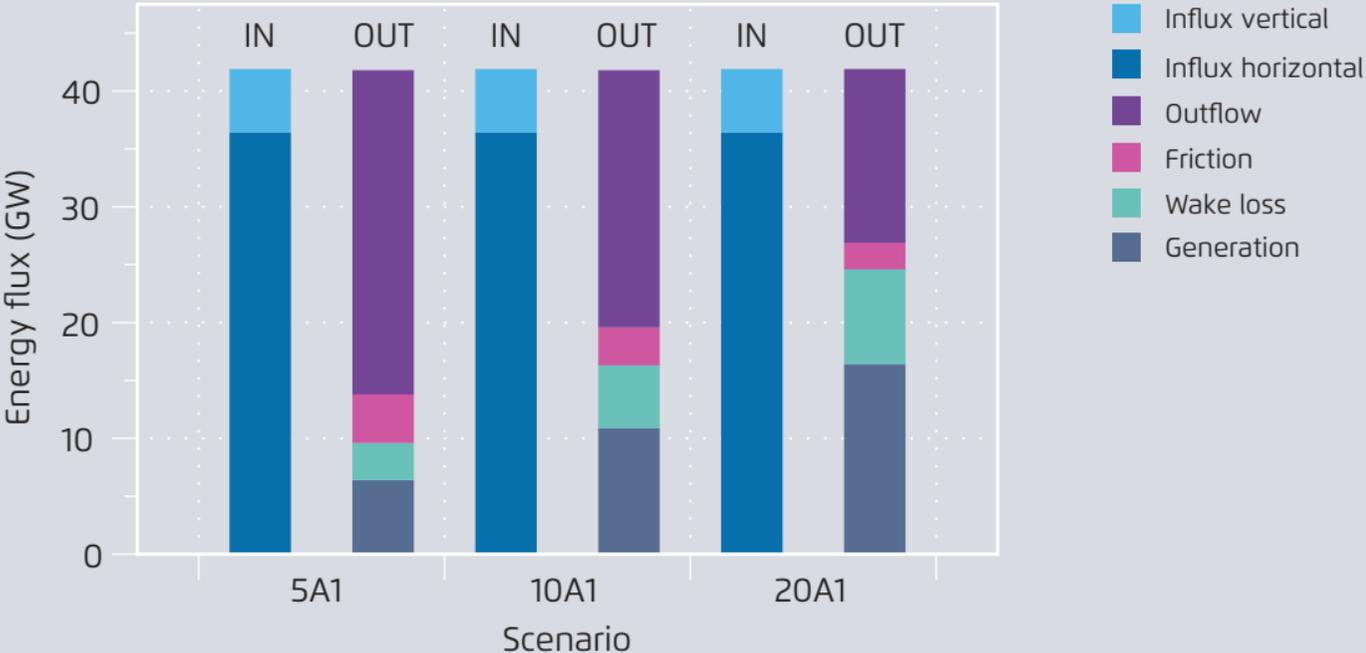
Influxes into the region as well as the share that is extracted by wind turbines (grey), that is lost by wake turbulence (turquoise) or surface friction (pink), or that leaves the region downwind (purple). The same colours are used for the arrows in the KEBA schematic diagram in Figure 7.
