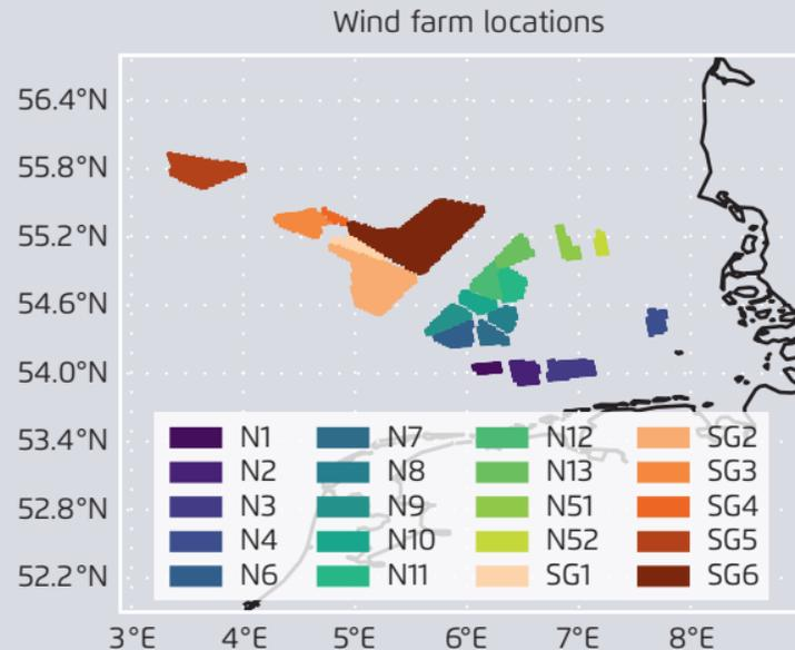
These two representations of wind farms are used in the mesoscale simulations and in the reference simulation without any wind farms. Each plotted coloured point represents a mesoscale grid box in which wind turbines are present.
