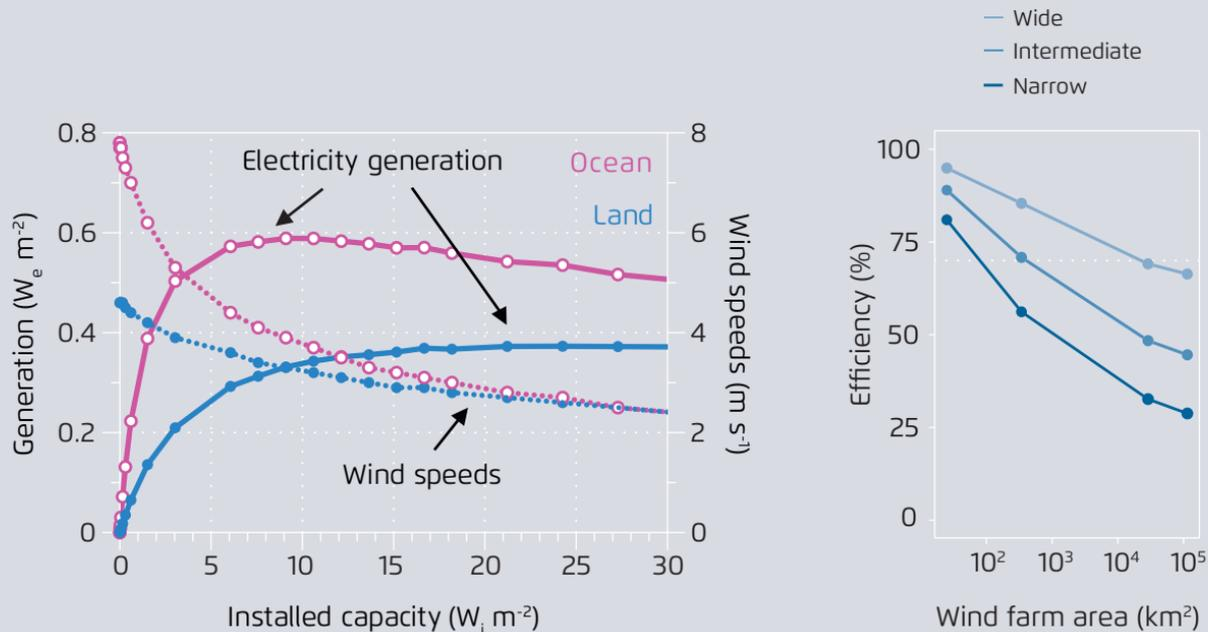
Left: Simulated electricity generation and mean wind speeds in idealized scenarios of complete coverage of the world with wind turbines of different installed capacities. The maximum generation results from reduced wind speeds at higher installed capacities. (Note that the maximum over land is broader than over the ocean and is reached at a higher installed capacity of  $25 W_i$  m<sup>-2</sup>.)
