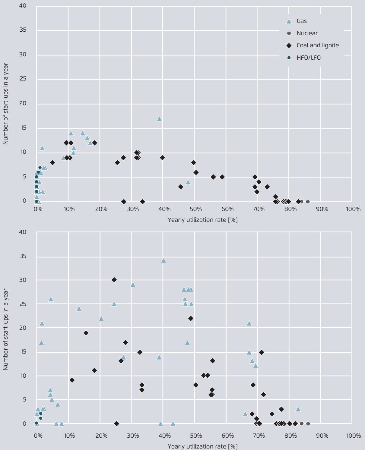
Yearly average utilization rates and number of start-ups (per year) on a unit level in the SEE region in 2017 (above) and 2030 (below)
