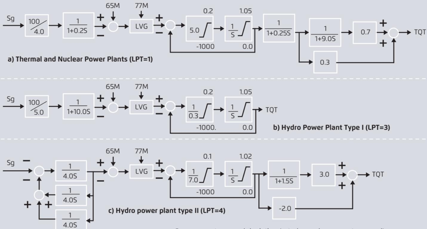
$Sg$  = generator speed deviation (rated speed – generator speed),
