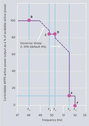
Note: (i) Droop is calculated with respect to registered capacity
