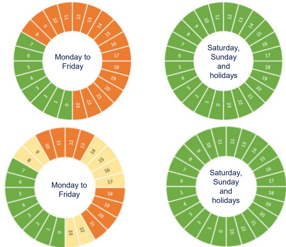
Figure: Power (upper diagrams), and consumption (lower diagrams) time periods for LV consumers with contracted power below 15kW.
